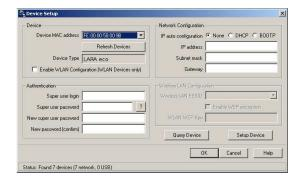
On the upper left corner, the MAC address of the LARA eco is displayed. To detect the MAC address manually, press the button "Refresh Devices". The displayed MAC address is the same MAC address printed on the white sticker placed on the back of the LARA eco. If the LARA eco is connected via USB, it is classified as an USB device and an appropriate drive letter is chosen for this device.
